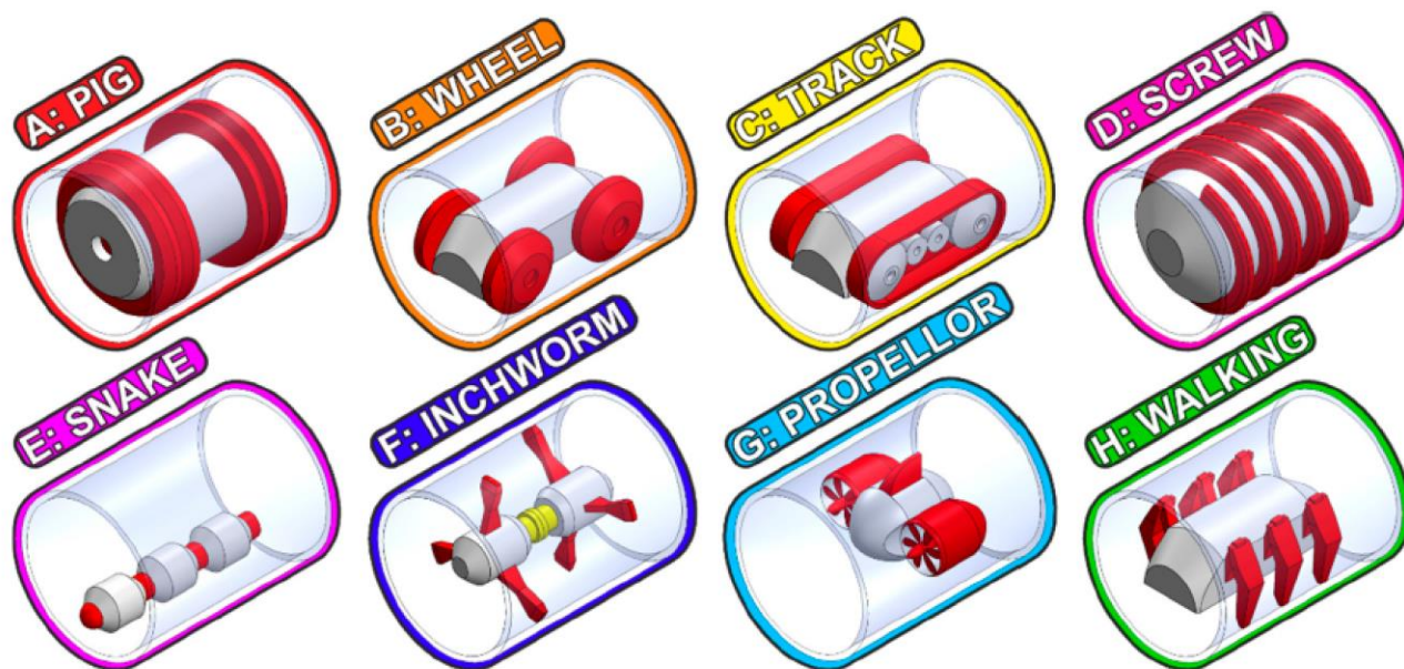
Fig. 9 –The eight main elements of in-pipe robotic devices `
